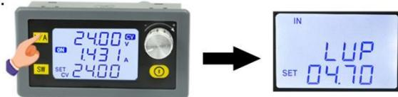
3.1>.At Normal Display Status, keep press **SW** button 2second enter into parameter set interface.
