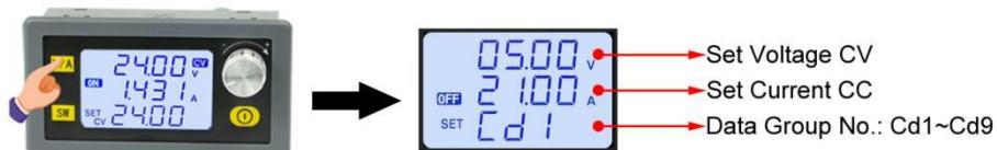
7.1>.This function is used to preset output voltage and current values, facilitating quick switching of output voltage and current values in the later stage. A total of 10 sets of parameter values can be set, and users can set commonly used values in advance.
