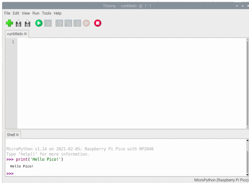
Figure 6. Saying "Hello Pico!" from the MicroPython REPL inside the Thonny environment.
