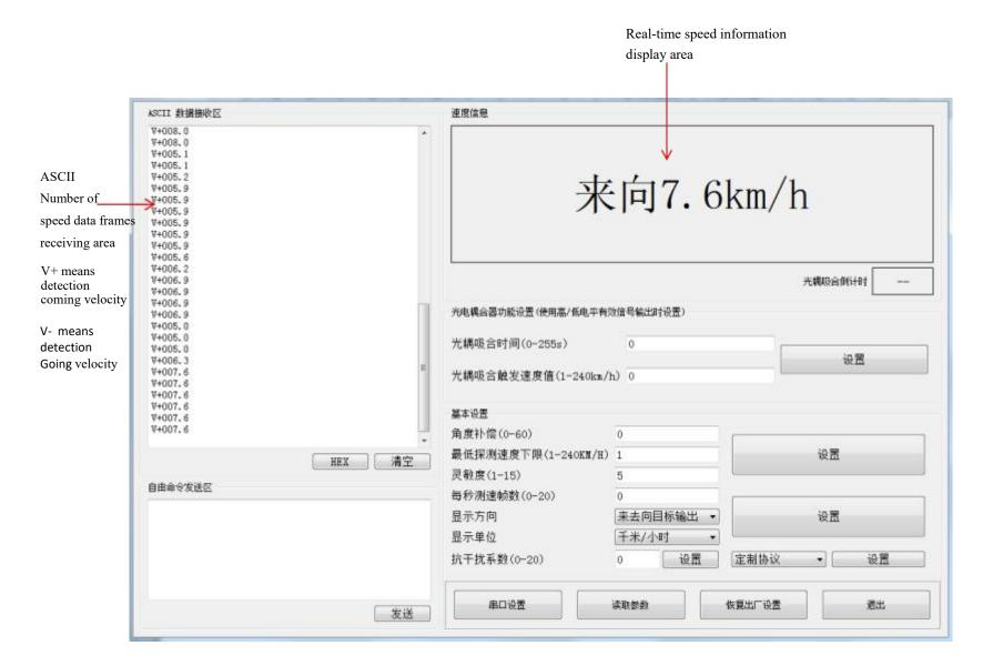
After the host computer is correctly opened and the radar is successfully connected, you can start using the host computer for debugging and setting parameters.
