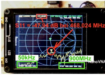
Now press the **Multi Function Switch** (MFS) to the right and hold it there. The marker moves from the start at 50kHz towards the higher frequencies. Try **f** = **468MHz**, it will show 468.042MHz. The display has a scale on the left hand side with 10dB divisions as well as the top "Zero dB point".
