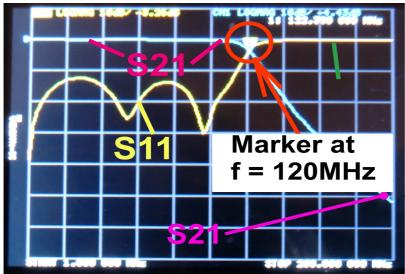
Note: The frequency marker can be moved using the MFS rocker action either left or right. All the data is shown at the top of the screen.
