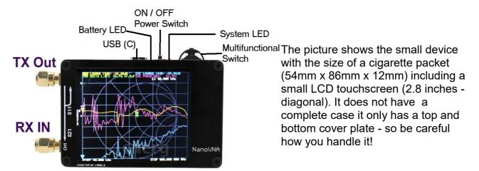
On the left there are of two SMA sockets: the RF input and output. The upper socket is the transmit port (CH0) and is the channel for S11 measurements (reflection). The lower socket is the receive input (CH1) and used for transmission measurements (S21).
