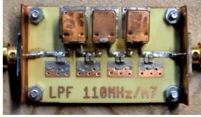
Since the current calibration is from 50kHz to 900MHz this is a good object to measure. The picture shows the test piece. It is a printed circuit board with SMA connectors attached using right angle copper sheets. The inner conductors of the SMA connectors form a low reflection connection on the central microstrip.
