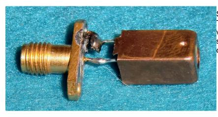
See the peparation: The coil (= an older Neosid version) is soldered to a SMA socket and then connected to channel CH0 of the NanoVNA.
