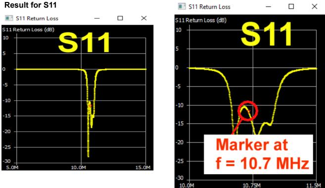
The left illustration uses a frequency range from 5....15 MHz, the right one from 10...11.5 MHz
