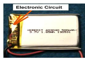
I have ordered one of these batteries on The Internet (6 Euros) and discovered that it contains a tiny circuit board. The test circuit shown was used
