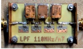
The SMA sockets are solded to two bended copper sheets. Thus the central conductor of the socket touches the central Microstrip Line and is then solded. This gives a transition with low reflection.
