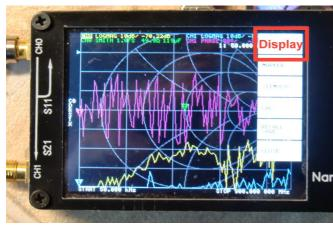
Leave the LOAD resistor on the TX port and tap on the screen with your finger or a "stylus" ("Stylus" = pen with rubber cap or a pencil fitted with small eraser).
