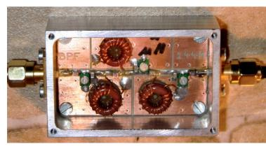
That is it! A Chebchev BPF with a centre frequency of 10.7 MHz, realised with Amidon ferrite ring cores (Q = 150).
