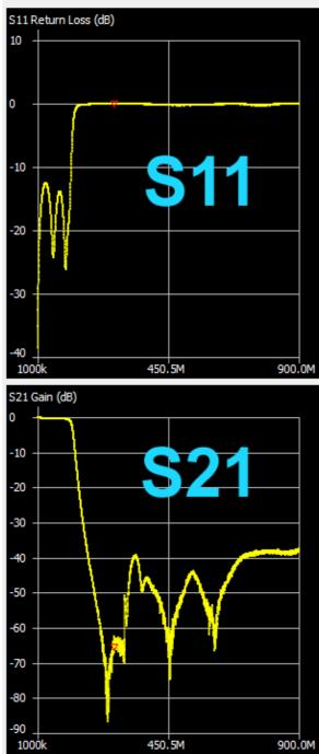
This is **S11 for the 50kHz to 900 MHz frequency range**. The **passband** can be identified without any efforts (= low reflection) and in the **stop band** we get a **total reflection with S11 = 0 dB**
