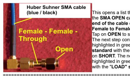
This opens a list that starts with OPEN. Attach the SMA OPEN calibration standard to the end of the cable connected to CH0 using the Female to Female coupler.
