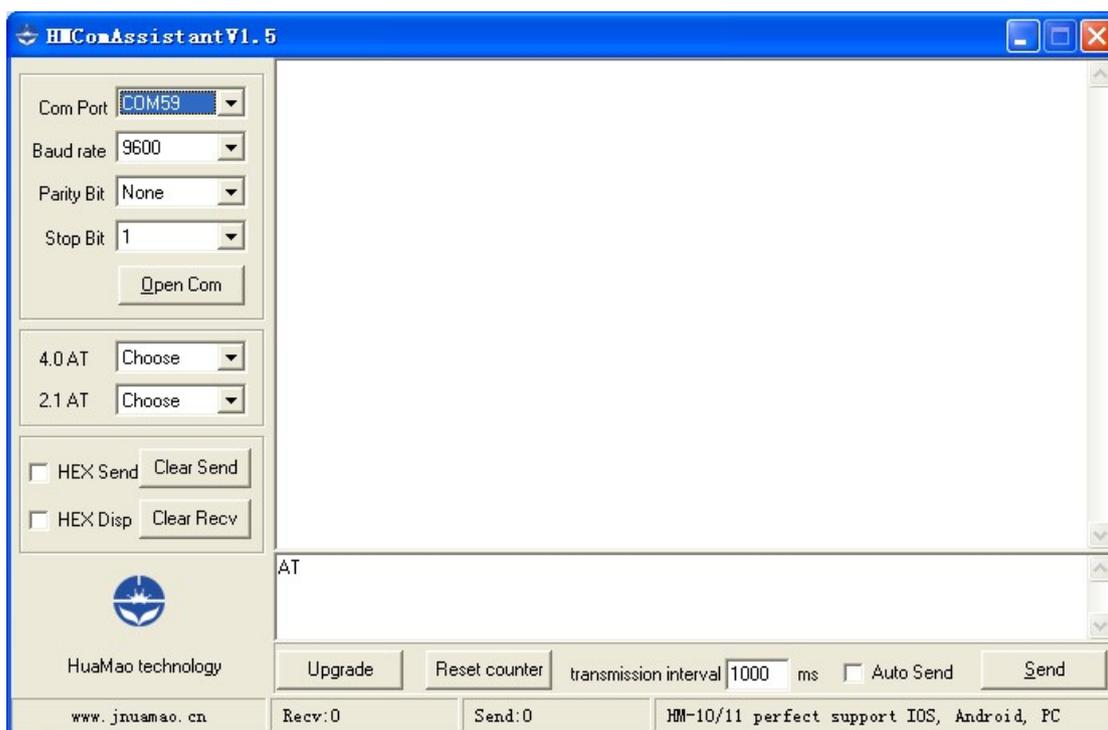
On Transmit version: module only accept AT Commands from UART interface when Bluetooth device is not connected with remote device.
